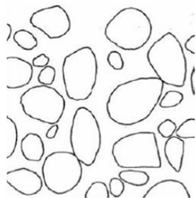
clean gravel framework
